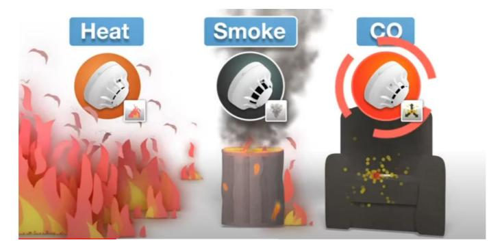
The 3OTech detector is programmed to constantly send information about the heat, smoke and CO levels in the room to the panel, which uses this information to help determine if there is a real fire. In this way it is able to more accurately determine the presence of a real fire and also reject false fire alarms caused by say dust or water vapour because the detector identifies smoke but not an increase in heat or CO.
