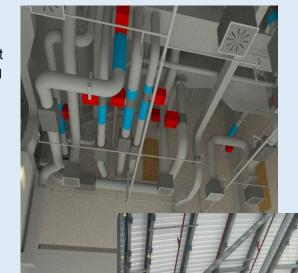
It is far easier and cheaper for the wall to be constructed first and to form the service penetrations. Also access was much safer with the services not in place
