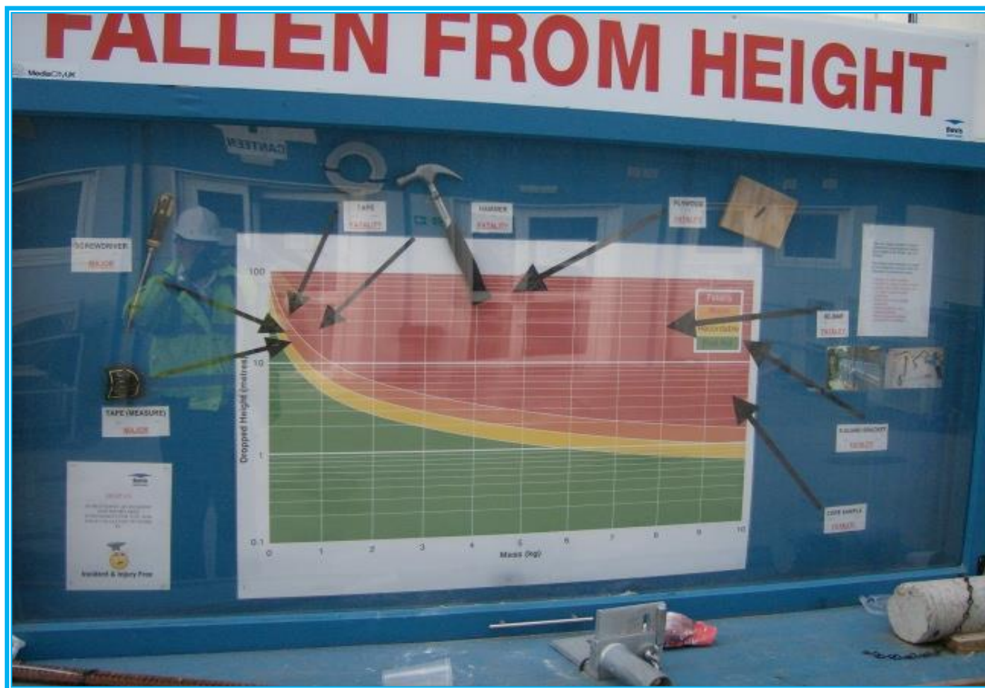
Site Notice Board Showing the Potential Implications of Various Falling Objects
