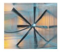
The machine can clean both rectangular and circular ductwork from 80mm diameter / square up to 900mm effectively. Re-sealable access panels (only 120mm diameter) can be cut into the existing ductwork up to 30m apart meaning access into the ceiling void / service risers of an existing building is limited. By using CCTV to inspect the ductwork before and after cleaning and to control the cleaning, where necessary, the entire process can be recorded for clients to keep to prove the cleanliness.
