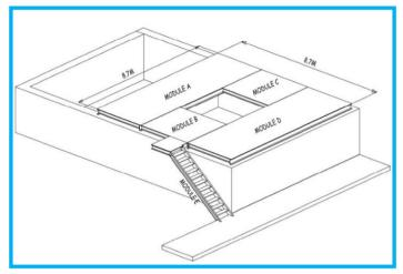
2 N° 8.0m x 8.0m platforms were split into 4 N° units that were built up offsite, delivered to site and connected together prior to the lift into the final position (Above and Right).
