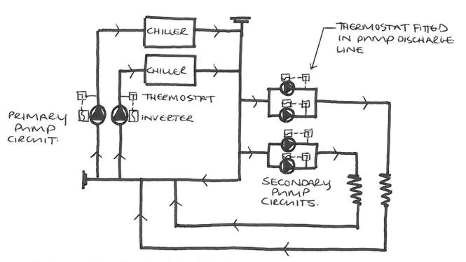
The thermostat would be hard wired directly to each pump inverter / starter i.e. not through the BMS, should the temperature rise above say 40°C then the pump would be automatically switched off. The thermostat should be positioned such that it cannot be isolated from the pump by closure of a valve. (An alarm could also be routed via the Building Management System to allow action by the plant engineer).
