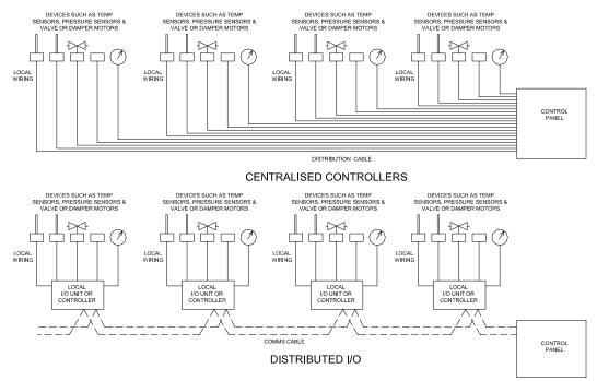
Distributed I/O is a system that places the input/output unit or controller very close to the field devices so that only local wiring is required. Typically a single I/O/controller would be positioned at each air handling unit, fan coil unit, underfloor heating manifold etc. Each controller would then be connected to each other and the control panel with a simple daisy chained communications cable, usually a twisted pair to the required specification.
