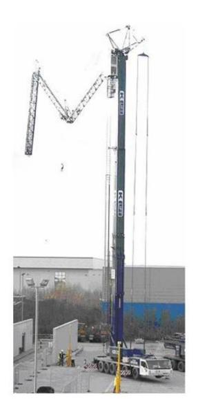
Rates (as at June 2006) range from £1600 to £2800 per day but this piece of equipment will be of particular advantage in situations where a normal mobile crane will not be able to operate due to the restrictions of adjacent buildings. It is also worthy of consideration where a mobile crane can be used but due to the stand-off distance a very large mobile crane would be required.
