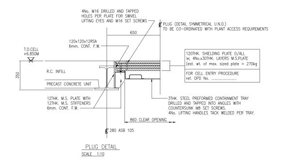
A plug detail was required for an access point in a reinforced concrete roof slab. The plug was required to provide containment and shielding. This detail utilises steel plate for the shielding with a separate tray to provide containment.
