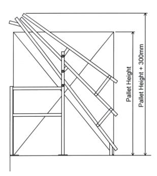
The solution was a Safety Barrier installation which allowed pallets to be safely loaded onto the mezzanine. A simple manual operation then allowed the steel barrier to be lifted over the pallets to protect the edge of the platform and allow access to the pallets at the upper level.
