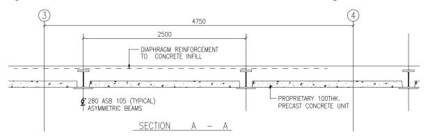
This detail eliminated the need for propping by using precast concrete (PC) units spanning between asymmetric beams, to support *in situ* concrete.
